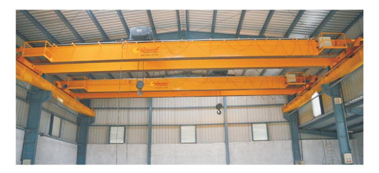
Ganesh heavy duty double girder cranes are designed and manufactured to customer's specific needs and suitable to end applications. We make double girder EOT crane up to 50 tone and 40 m span.
